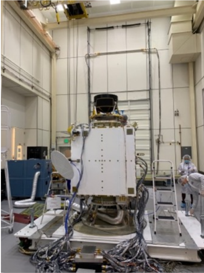
Above: Close out of two of DART spacecraft panels
