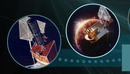
**LES 8\*** Mar. 14, 1976–2004 2 MHW RTG: 158 W<sub>e</sub> BOL **LES 9\*** Mar. 14, 1976–2020 2 MHW RTG: 158 W<sub>e</sub> BOL **Voyager 2** Aug. 20, 1977–Present 3 MHW RTG: @~158 W<sub>e</sub> BOL
