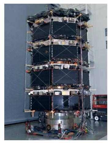
**TOP:** The four MMS spacecraft are stacked in preparation for vibration testing. *Image Credit: NASA/GSFC*
