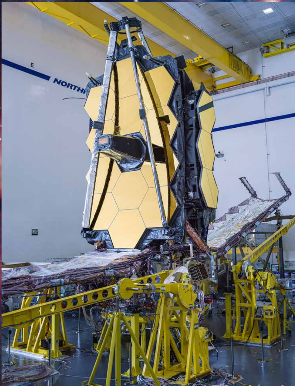
The Webb observatory in the clean room in Redondo Beach, CA in August 2019 before observatory environmental testing and observatory deployment tests
