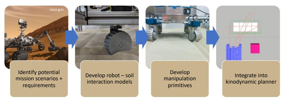
Current project: use robot-soil interaction models to gain NPTM-specific rover design insights
