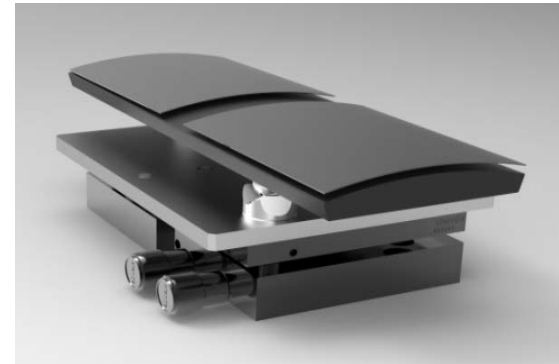
Mirror module containing one pair of parabolic-hyperbolic mirror segments 50X thinner than Chandra's.
