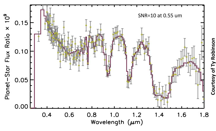
SNR=10 at 0.55μm 10<sup>-10</sup> raw contrast Constant 30% throughput Integration time *per* bandpass
