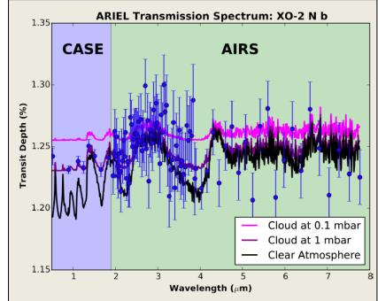
CASE breaks the degeneracy between clear and cloudy atmospheres present at longer wavelengths. The blue dots are simulated, single-transit observations by CASE and AIRS, the two ARIEL instruments. Both instruments observe the object simultaneously. The target is a hot Jupiter planet with simulated clouds at 1 mbar.
