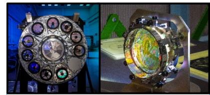
The Wide flight Element Wheel Assembly (EWA) is complete, installed, and aligned in the instrument at Ball
