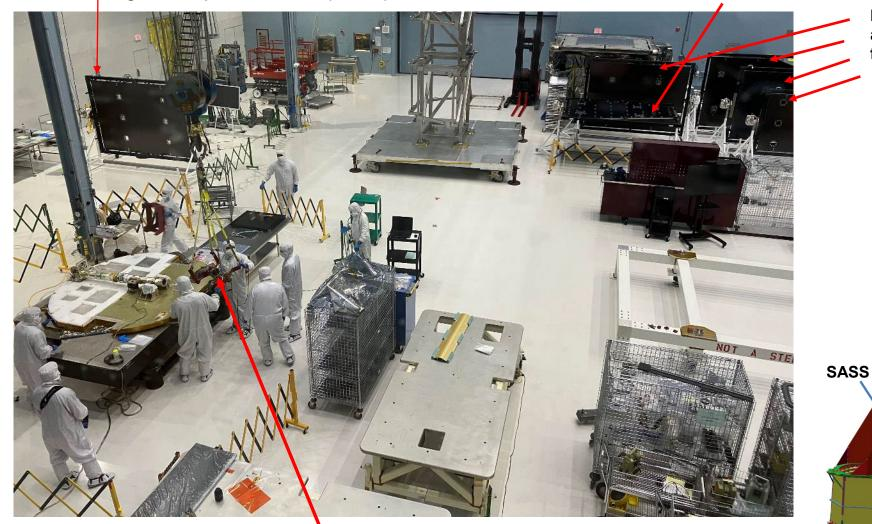
Gimbal actuator Flight assembly being lifted onto the High Gain Antenna System (HGAS) Communication Panel for a fit check prior to match drilling Solar Array Sun Shield (SASS) Shown on Observatory – see right
