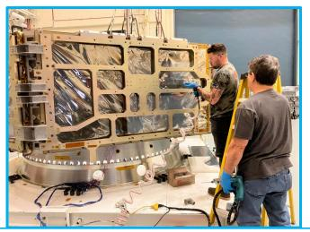
Match drilling of bus to avionics panels in B.29 High Bay
