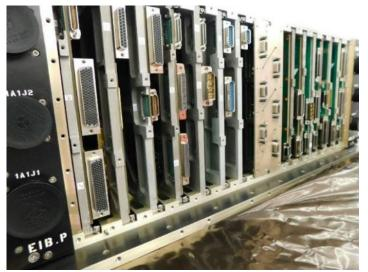
Telescope Control Electronics (TCE) Module Complete
