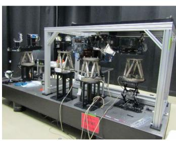
Tertiary Optical Mirror Assembly (TOMA) Mirror Integration and Alignment. Enhanced the Tip Tilt Fold Assembly (TTFA) actuator to comply with GSFC standard practice
