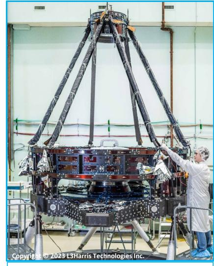
Forward Structure Assembly (FSA) successfully integrated to Primary Mirror Assembly (PMA) ★ Heritage Hardware Complete ★
