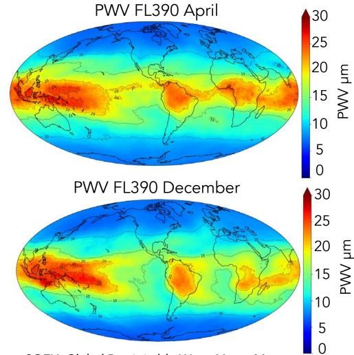
SOFIA Global Precipitable Water Vapor Maps Mission has developed tools to forecast water vapor anywhere in the world
