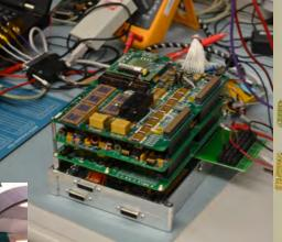
**Particles & Fields** Data Processing Unit (PFDPU) **Partial Stack**
