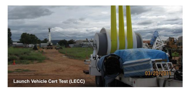
CSBF completes Launch Head Certification "drop test" at the specified qualification load of 3600lbs prior to the LECC.
