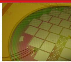
100 mm diameter flat Eagle test mirror (PZT electrode cells, printed electrode contacts, and strain gauge patterns, used for diagnostics).
