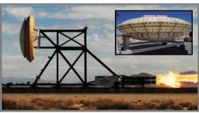
Low Density Supersonic Decelerator Sled Test
