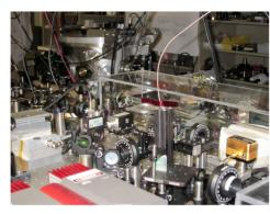
lodine laser stabilization setup and cavity
