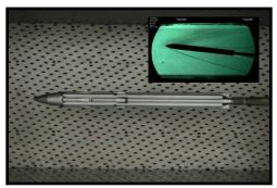
SWORDS model for wind tunnel testing at NASA MSFC
