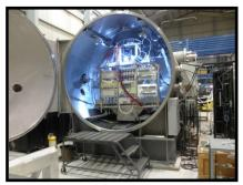
Nuclear Systems delivered the Fission Power System Technology Demonstration Unit (TDU) Reactor Simulator
