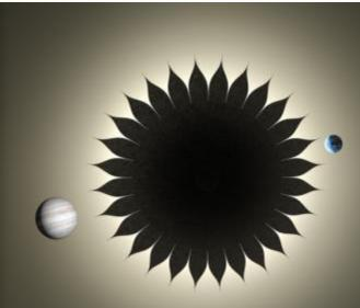
The starshade probe-class mission is the only way to reach down to rocky exoplanets with a relatively small space telescope
