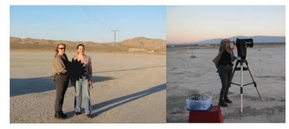
Desert field testing at 1% scale has demonstrated contrasts at 10<sup>-7</sup>; Glassman et al. 2013
