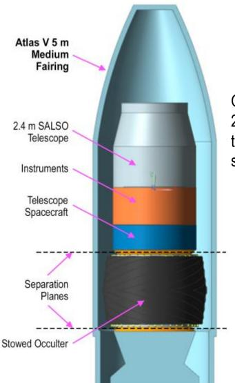
Occulter with 2.4-m NRO telescope stacked on top
