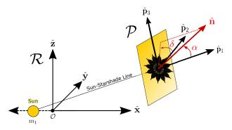
FIGURE 57. Diagram of the  $\mathcal{R}$  and  $\mathcal{P}$  frames used in the starshade equations of motion. The  $\mathcal{P}$ -frame is defined perpendicular to the Sun-Starshade vector. Based on Dachwald et al. (2006). From Soto et al. (2019)
