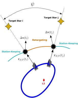
FIGURE 58. Schematic of the two starshade flight modes: station-keeping with star i, retargeting to a star j, and station-keeping with star j. An angle  $\psi$  separates the LOS vectors to the two stars. From Soto et al. (2019).
