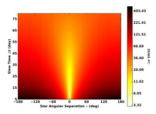
FIGURE 59. Heatmap of  $\Delta v$  as a function of both star angular separation  $\psi$  and slew time  $\Delta t$ . Interpolated values are shown. Colorbar is shown in log-scale. From Soto et al. (2019).
