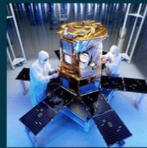
SORCE is 290 kg based on an Orbital LEOSat-2 bus
