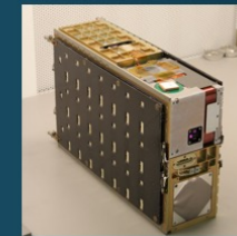
CSIM is 11 kg based on a Blue Canyon Technologies bus
