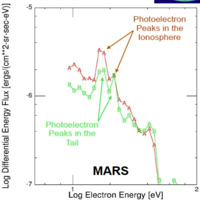
Peaks in the electron spectrum are cause by solar HEII 30.4 nm ultraviolet light ionizing carbon dioxide and atomic oxygen in the atmosphere. The emitted electrons are observed in the dayside lonosphere near the ionization source; however, they are also observed deep in the planet's tail traveling away from the Sun. This proves that the atmospheres of both Mars and Venus are being stripped away in an ionization process caused by the Sun.
