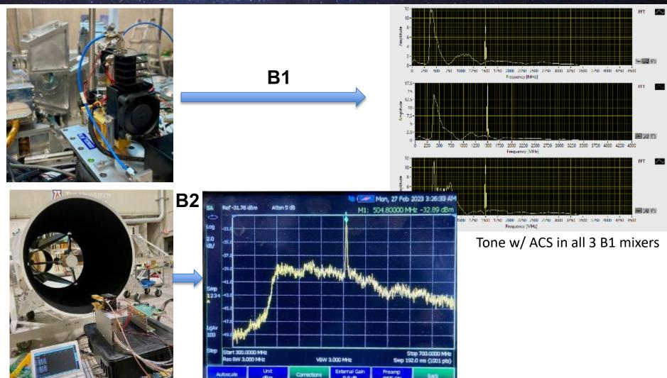
End-to-end tone tests provide strong evidence that GUSTO is fully functional
