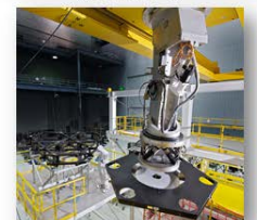
Primary Mirror Segment Assembly (PSMA) Installation Fixture (PAIF)
