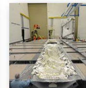
Sunshield Deployment Testing
