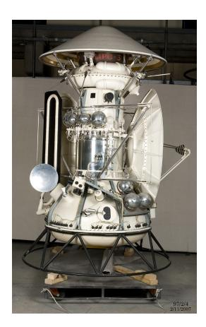
FIGURE 2.3 A full-scale model of the Mars 3 orbiter and lander. SOURCE: Collection: Museum of Applied Arts and Sciences. Photo: Nitsa Yioupros.
