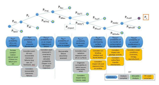
**FIGURE 3.6** A schematic depiction of the Icy Bodies Planetary Protection Probabilistic Model used to calculate the probability of icy body contamination. SOURCE: Redrafted from an original provided by the Europa Clipper Project, NASA, Jet Propulsion Laboratory
