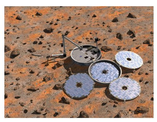
**FIGURE 2.5** An artist's impression of how Beagle 2 should have unfolded itself to deploy its instrumented arm, solar panels, and main antenna once it had landed on Mars. It is believed that various petals did not fully deploy upon landing. SOURCE: European Space Agency, "Artist's Impression of Beagle 2 Lander," January 23, 2002, http://www.esa.int/spaceinimages/Images/2001/04/Artist\_s\_ impression\_of\_Beagle\_2\_lander. Courtesy of European Space Agency/Denman Productions.
