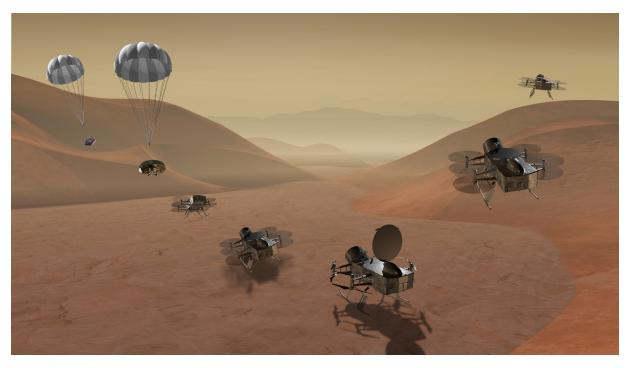
**FIGURE 3.8** An artist's conception of Dragonfly, a rotorcraft lander designed to explore Titan. It is currently under study as one of two possible candidates for NASA's fourth New Frontiers mission for launch in the mid-2020s. SOURCE: Courtesy of Johns Hopkins University Applied Physics Laboratory/Steve Gribben.
