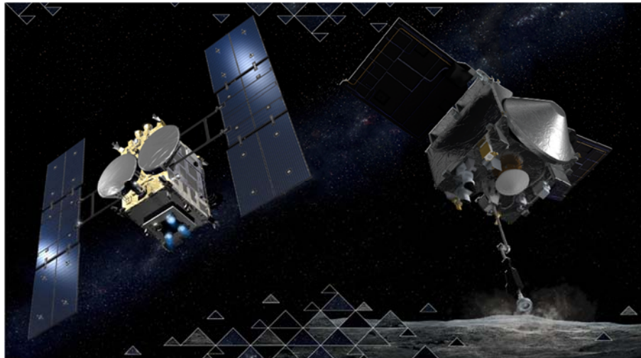
FIGURE 3.1 Dual asteroid explorers: Left: Artist's rendition of Hayabusa2 (JAXA) Right: Artist's rendition of OSIRIS-REx spacecraft performing a 'touch and go' sample acquisition at Benu. SOURCE: From the Bruce Murray Space Image Library of the Planetary Society. NASA / Goddard / University of Arizona / JAXA 2
