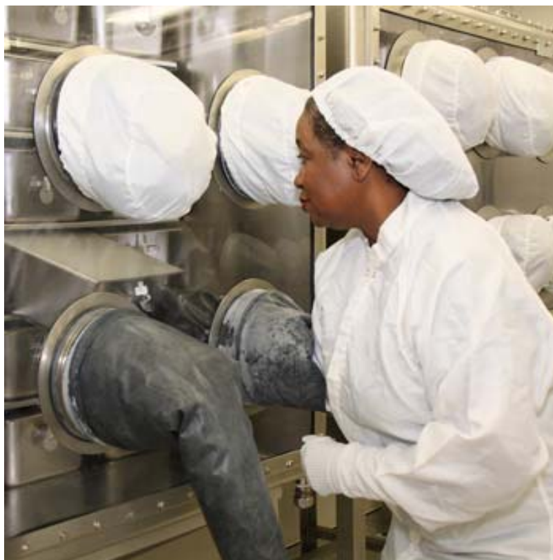
FIGURE 4.2 A lunar sample processor prepares to begin work on pristine lunar samples by placing her hands in the gloves attached to a nitrogen-filled glovebox. SOURCE: https://curator.jsc.nasa.gov/lunar/laboratory_tour.cfm
