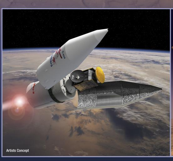
Separation of the payload fairing during launch sequence
