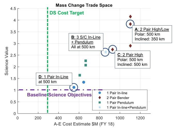
In Pre-Phase A, further refinements have led to: Architecture D: Baseline concept for MC (NASA/DLR) Architecture B and C: Eliminated Architecture A: Possible; combination of MC and NGGM (ESA)
