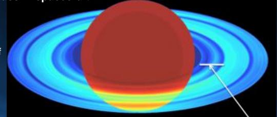
The output brightness temperature map generated from Cassini RADAR data. Red is hotter material, blue is colder.
