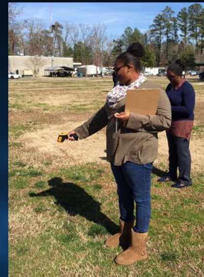
Above: Student from Elizabeth City State University demonstrates how to use an Infrared Thermometer to measure Surface Temperature.
