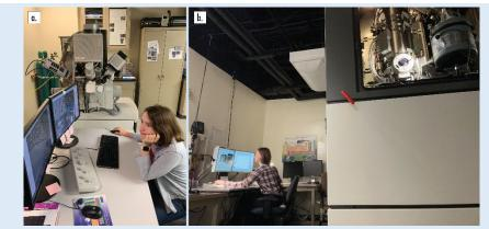
Figure Caption: AEMC researchers using (a) the dual-beam focused ion beam scanning electron microscope (FIB/SEM) and (b) the scanning / transmission electron microscope (S/TEM) in the AEMC facility.
