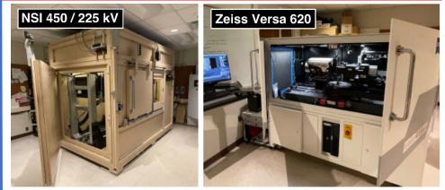
**UTCT XCT Scanners**. (left) NSI scanner: 450- and 225-kV X-ray sources and a flat-panel detector for larger and/or relatively more attenuating samples. (right) Zeiss Versa 620 scanner: 160-kV X-ray source and six detectors for smaller and/or relatively less attenuating samples and DCT.
