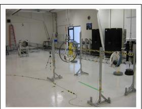
GOES-R MAG instrument fully deployed. Credit: NOAA
