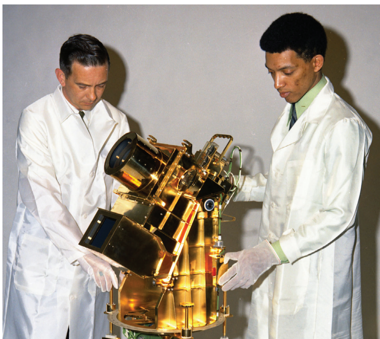
Born in 1939, George R. Carruthers [right] developed the Far Ultraviolet Camera/Spectrograph, the first Moon-based telescope. Carruthers and William Conway , a project manager at the Naval Research Institute, examine the gold-plated telescope, used during the Apollo 16 mission to make the first observations of Earth from a distance in ultraviolet (UV) light, showing the full extent of the hydrogen atmosphere, the polar auroras, and the tropical airglow belt. In 1970, Carruthers made the first detection of molecular hydrogen in space using a sounding rocket. He has also worked on UV imaging of Earth's polar auroras and of the faint photochemical luminescence found in the upper atmosphere. Photo credit: U.S. Naval Research Laboratory
