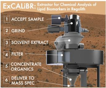
**Figure 2:** ExCALiBR instrument uses 5 sample processing steps to provide a mass spectrometer with unadulterated, concentrated lipids from Martian regolith. ExCALiBR can be deployed to characterize the origin of organics on Mars.
