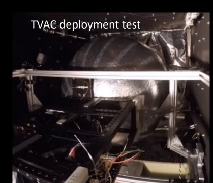
Deployable line feed for frequencies from X-band
