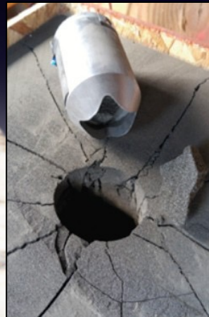
Sampler test: 14.6 cm penetration in 2.4 MPa material
