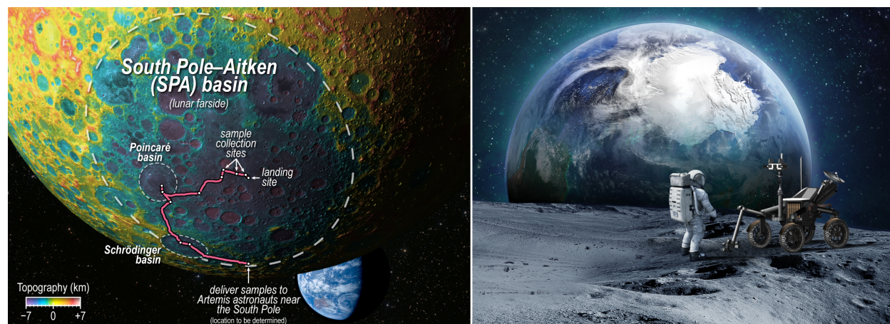
Figure 1: The Endurance concept. Left: the baseline Endurance traverse. The rover would traverse ~2,000 km from the center of SPA to the south pole, collecting ~100 kg of samples from 12 key sites along the traverse. Right: An artist concept of the rover rendezvousing with Artemis astronauts at the south pole. Figures adapted from the Endurance concept study report. The full Endurance report is publicly available: tinyurl.com/2p88fx4f .
