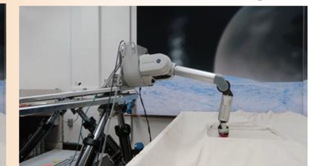
A demonstration showing how the lander's legs can get lifted off the surface when carrying out a pressure sinkage test in the low gravity of Enceladus
