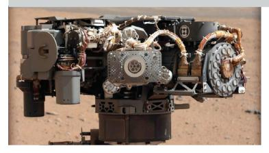
Developed for the Mars Science Laboratory Mission, the Alpha-Particle X-Ray Spectrometer (APXS) is a contact instrument that uses X-ray spectroscopy to determine the elemental composition of soils and rocks. The science objective of the APXS is to produce an understanding of the formation, evolution, and biological potential of the landing site environment through analysis of the variations in elemental composition and distribution of elements comprising the Martian materials.
