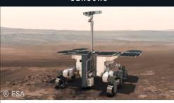
MDA provided the electromechanical components required for all on-surface rover locomotion and deployment after landing. These operations are enabled through the use of BEMA's 18 active DOFs which are enabled via 3 bogies, each connected to a wheel pair. All wheels can be pivoted to adjust the rover height and angle with respect to the local surface, and to provide walking ability, particularly useful in soft, non-cohesive soils like dunes.
