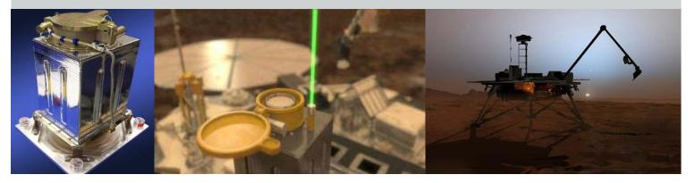
MDA developed the Meteorology package (MET) on the Phoenix Mars Lander, to provide characterization of the Martian climate. The MET consisted of a lidar, three thermocouples and a pressure sensor.
