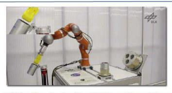
Exhibit E. Stage 5a – Handling: SARP Inspection and Removal (Ground Command). A ground-commanded sequence takes a set of inspection images. Once downlinked and reviewed, a ground-commanded sequence has the RA grasp the KINEE interface and remove the SARP from the Inner Sheath. The STS is robust to multiple failures. (Above figure shows the DLR prototype arm removing the SARP during end-to-end testing [§J.10.6.2.2].)
