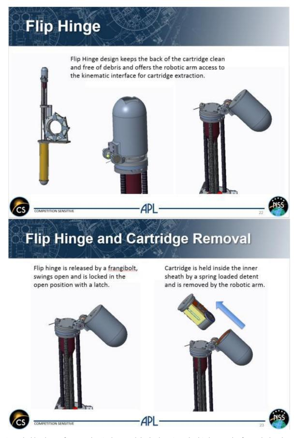
The SARP is reeled back to a firm mechanical ground, locked against the birdcage. The frangebolt releases the flip hinge exposing a clean interface for the KINEE. The clean sample cartridge is extracted from the SARP by the robot arm.
