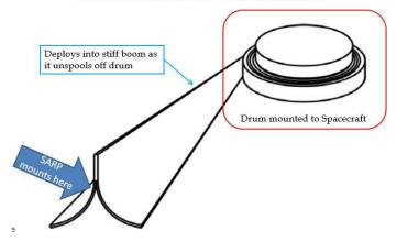
Visualization of the TRAC boom rolling flat on the reel but deploying to generate a more rigid cross sectio
