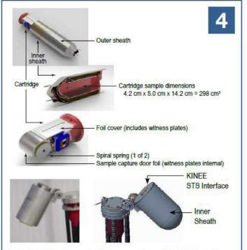
Exhibit D. Stage 4 – Preparation: SARP Rotation (T=21 s). A final timer actuates the flip hinge, rotating the Cartridge and Inner Sheath away from the TRAC boom decoupler plate and exposing the KINEE interface.
