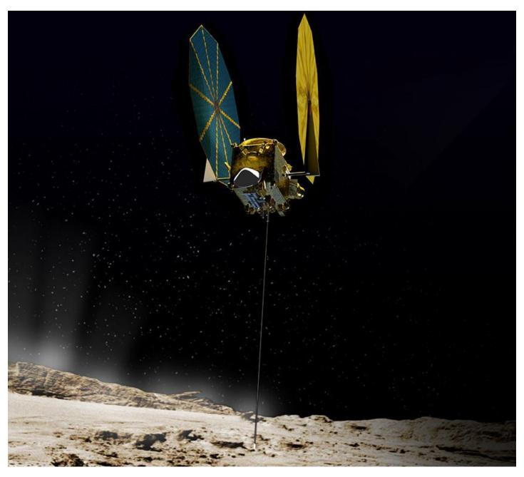
Deployment: SARP launch and sample collection at a comet. The CORSAIR spacecraft commands the launch of the SAS at 10 m. The Launcher accelerates the SARP to penetrate >10 cm into the surface. The SARP Outer Sheath bears the impact forces and breaks up material for ingestion. Under-dense material is compressed to fill the cartridge. The SARP comes to rest through comet resistance, retraction system braking, or both.
