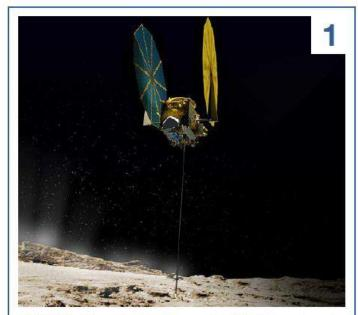
Exhibit A. Stage 1 – Deployment: SARP Launch and Sample Collection (T=0; Launch). The SC commands the SAS at 10 m. The Launcher accelerates the SARP to penetrate >10 cm into the surface. The SARP Outer Sheath bears the impact forces and breaks up material for ingestion. Under-dense material is compressed to fill up the cartridge. The SARP comes to rest through comet resistance, retraction system braking, or both.
