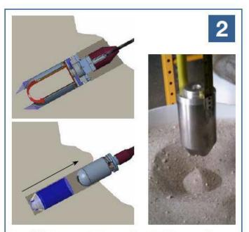
Exhibit B. Stage 2 – Acquisition: SARP Door Close and Decouple (T=1–2 s). A timer closes the Cartridge door, cutting through material and fully encapsulating the sample. Another timer separates the Outer Sheath from the Inner Sheath, providing a well-understood friction force for removal. (Right figure shows SARP testing.)
