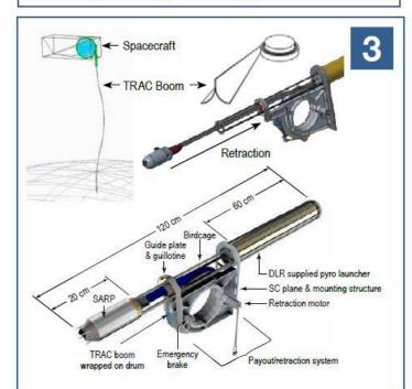
Exhibit C. Stage 3 – Retraction: SARP Return (T=2–11 s). The Boom Retraction and Deployment (BRAD) controls the SARP return to the end of the Launcher to avoid buckling. The SARP is mechanically grounded at the end of the launcher. The ADAMS model was used to analytically verify buckling margins.
