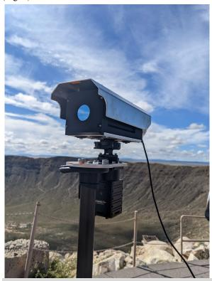
**Figure 1:** One of two PORIS prototypes, here fielded at Meteor Crater, AZ. The 1 lb. instrument is mounted on a tripod (out of view to the bottom), and includes a compact scan motor controlled by a tablet computer that also collects and processes the hyperspectral data.
