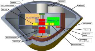
Figure 1. Preliminary Saturn Probe Design Preliminary Mass Estimate of this concept is 135.8\* kg including 30% reserve. Preliminary Cost Estimate (FY20\$): \$94M including 30% reserve.
