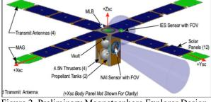
Figure 2. Preliminary Magnetosphere Explorer Design
