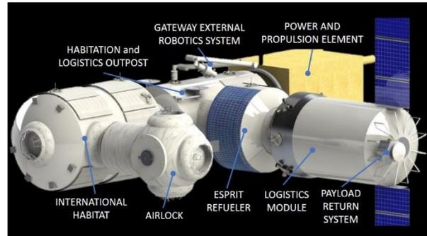
**Figure 1: Planned Gateway elements showing Logistics Module with attached small spacecraft-based payload return system.**
