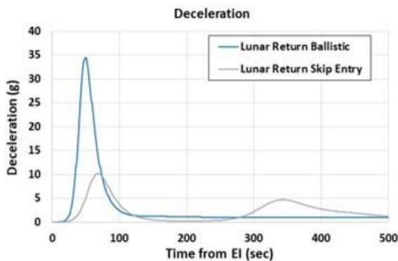
**Figure 9: Deceleration load comparison between ballistic and guided blunt body entry systems.**
