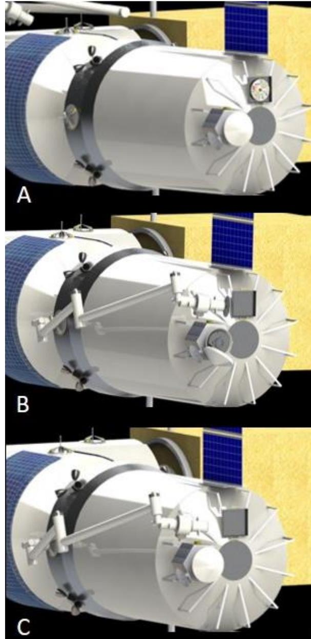
**Figure 5: Transfer operations of externally exposed samples transferred into the SSRS using the robotic arm.**
