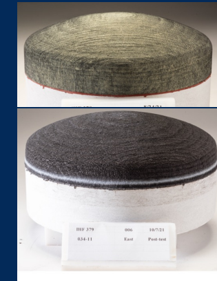
2021 era instrumented thermal response models used to develop material model for TPS sizing
