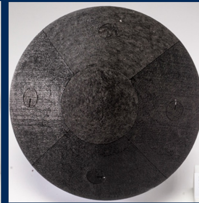
SPRITE model geometry allows assessment of a range of conditions and rapid evaluation of material capability including material compositions and seam designs (Flank heating ~400 W/cm 2 , shear ~ 200Pa on flank and ~500Pa on shoulder)
