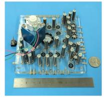
*Figure 1.* SPLIce 1.0 prototype with integrated liquid-handling components. Dimensions: 16 x 15 cm.
