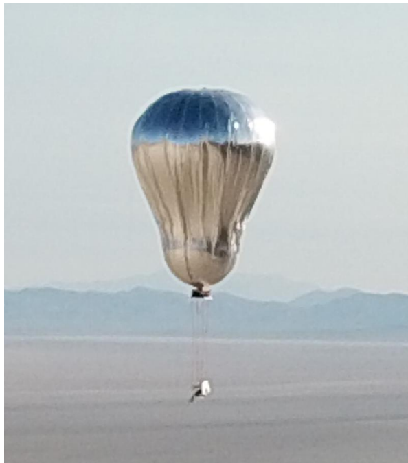
Figure 1 One-third scale variable altitude aerobot under test in the Black Rock desert in Nevada in July 2022. Exchange of helium between an inner and an outer balloon is used to change the buoyancy of the vehicle and execute altitude changes. (J. Izraelvitz, JPL)
